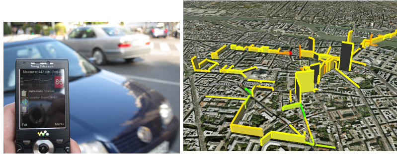
Fig. 1 The NoiseTube project [8]. A sensing project mixing mobile sensing applications with participatory and community building aspects to create a collective exposure map of noise pollution.
